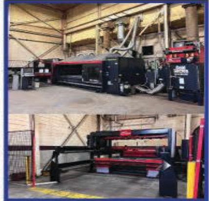
4000 Watt Amada FO MII 3015NT Laser with MP Flexit Sheet Loader New: 2013
